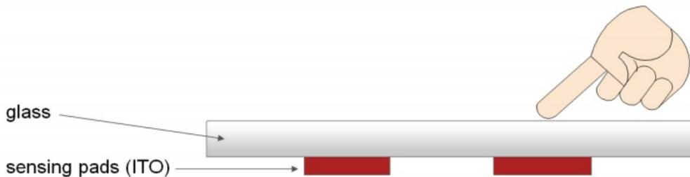
**Figure 4.5:** Capacitive touch screen consisting of one ITO layer. (Fischer 2010)
