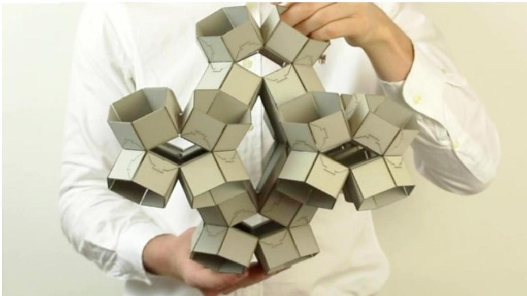
**Figure 2.37:** A reconfigurable foldable structure. (Overvelde et al. 2017)
