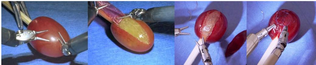
**Figure 3.5:** The technology used to suture a tiny grape helps perform delicate and minimally invasive surgery. [Source: DaVinci Surgical System]
