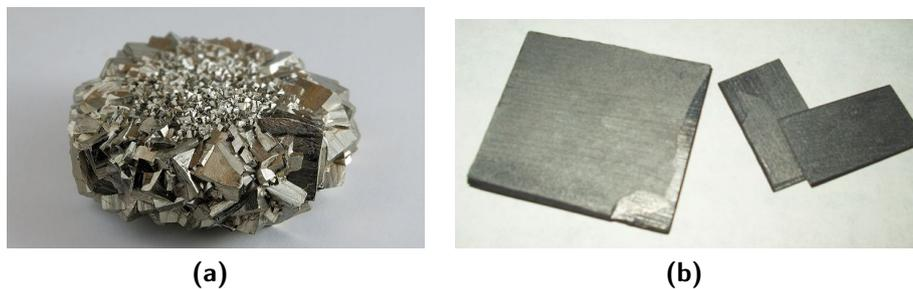
**Figure 1.4:** a: A mass of intergrown pyrite crystals. b: Sheets of pyrolytic carbon. [Source: worldatlas,wikipedia]
