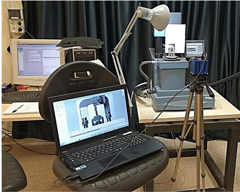
**Figure 5.21:** Camera set-up for the auxetic test.
